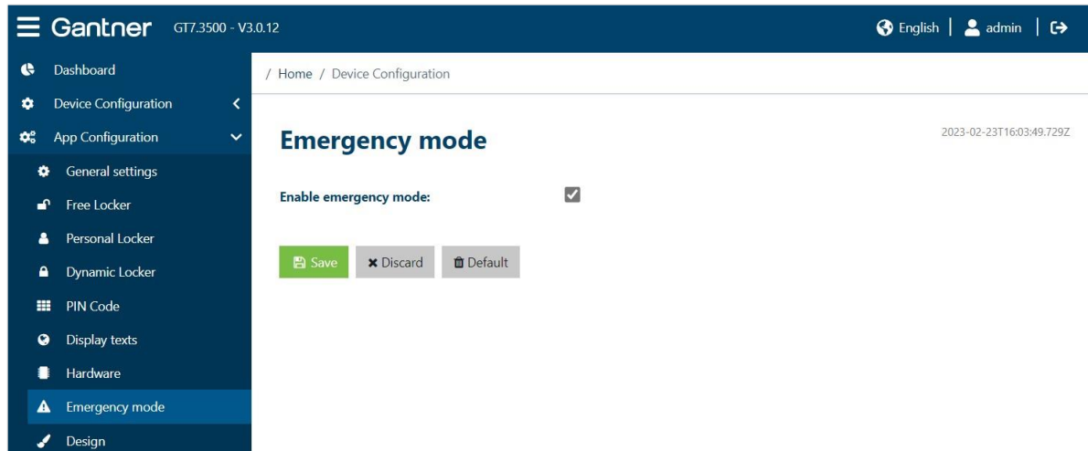
Figure 4.34 – GT7 Central Locker web interface – Emergency mode
