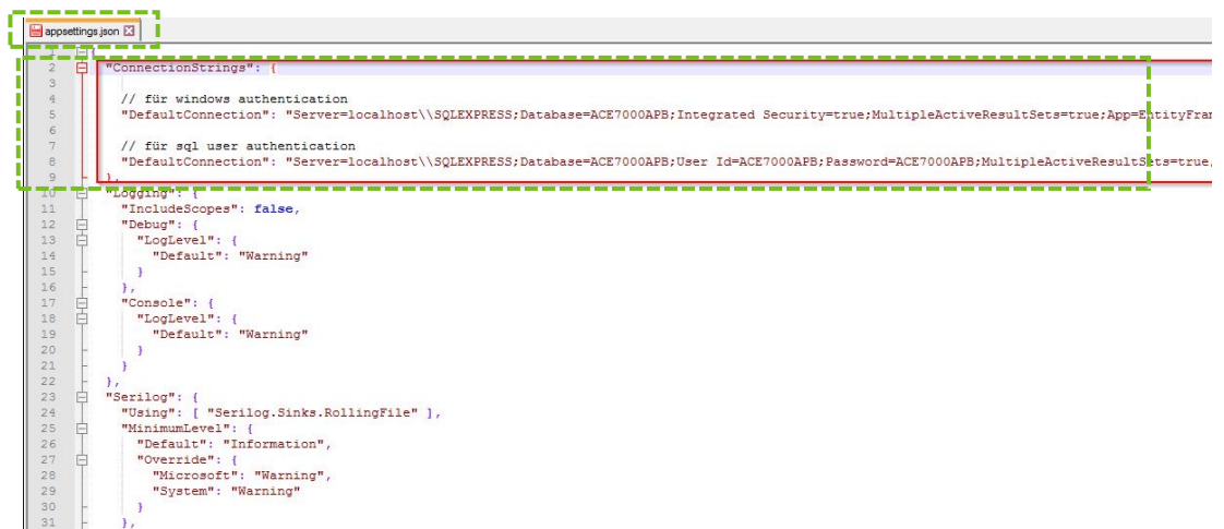
Figure 3.15 - Server connection data in the “appsettings.json” file
