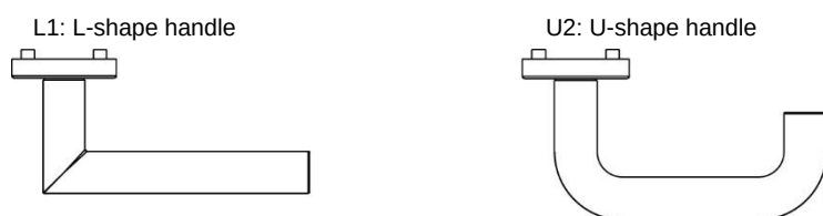
Figure 2.2 – GAT DL 34x handle shapes
